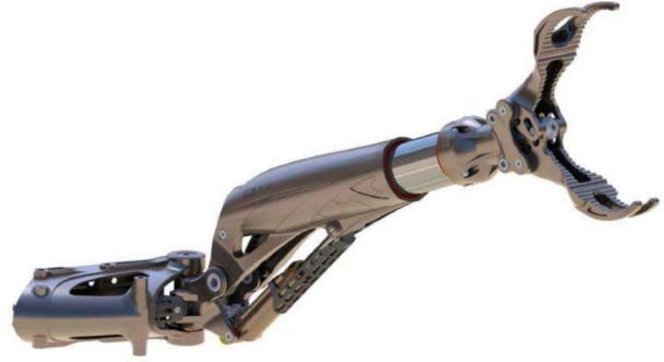
The TitanRob G501 is a five-function hydraulic grabber manipulator made of titanium and developed for Observation- and Light Work Class ROVs. It is a manipulator with enhanced characteristics of weight/power ratio and capabilities: by using titanium as main material, lower weight and more mechanical characteristics are achieved which allows for improved dimensioning.
