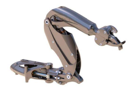
The TitanRob M501 is a five-function hydraulic manipulator made of titanium and developed for Observation- and Light Work Class ROVs. It is a manipulator with enhanced characteristics of weight/power ratio and capabilities: by using titanium as main material, lower weight and more mechanical characteristics are achieved which allows for improved dimensioning.
